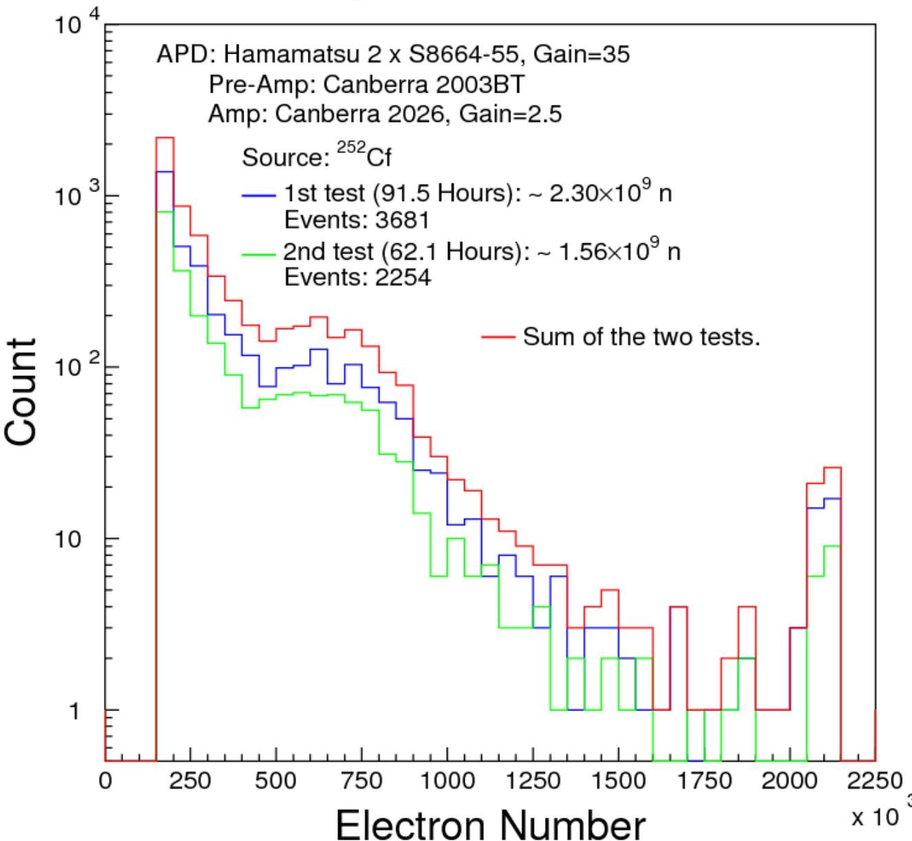
Data were taken with the SA gain at 2.5. The up-limit of the pulse height distribution is  $\sim 2$  M electrons, or 7.2 MeV deposition in APD, which corresponds to 1000/ 500 GeV, assuming the light yield is 2/4 p.e./MeV.
