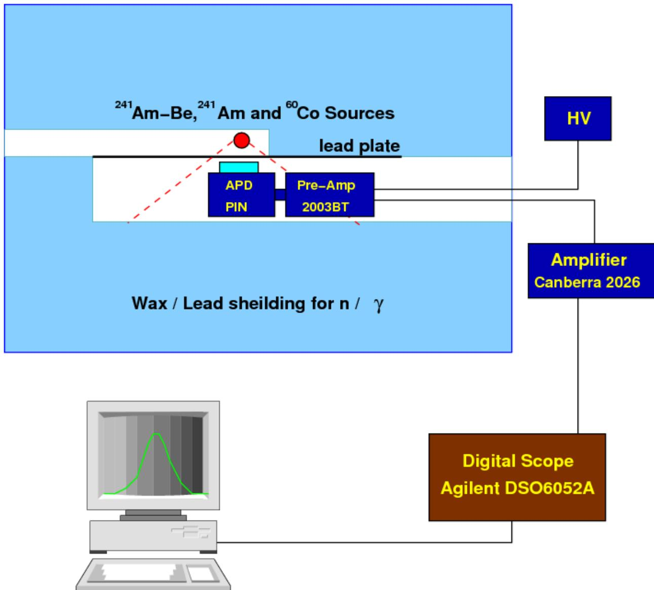
Si APDs/PIN were placed at 2 cm from several sources:  $^{241}\text{Am-Be}$ ,  $^{241}\text{Am}$  and  $^{60}\text{Co}$  with the neutron and  $\gamma$ -ray flux of  $6 \times 10^4$ ,  $1.06 \times 10^7$  and  $1.54 \times 10^6$  /cm<sup>2</sup>/s.
