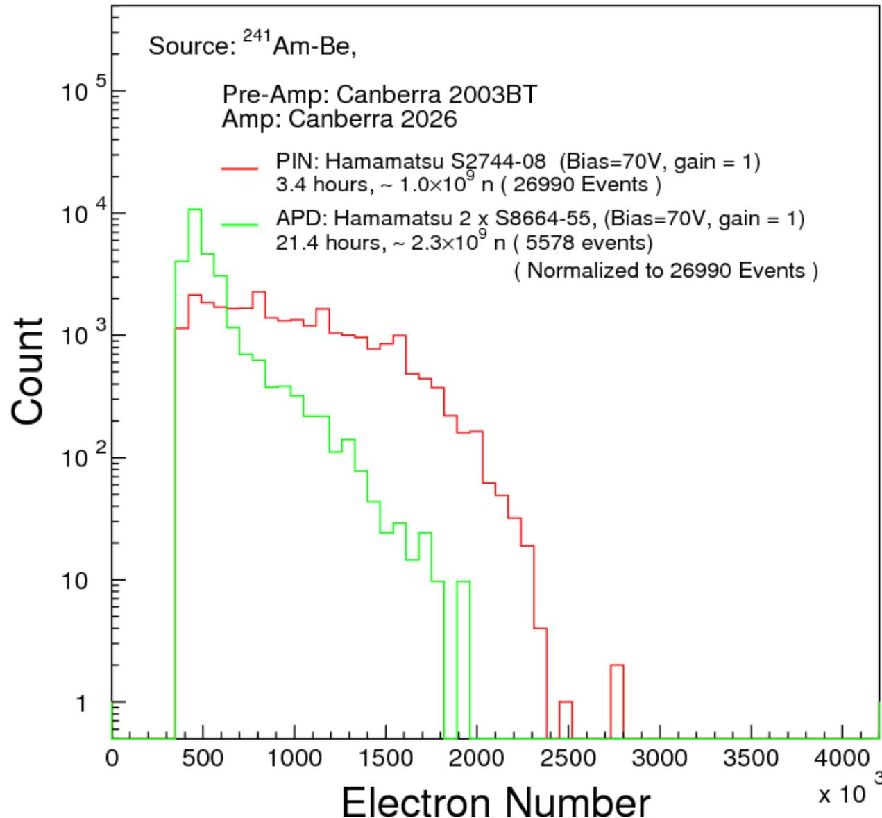
Signals of up to 2.5 and 2 M electrons were observed in the PIN and APD with unit gain respectively, corresponding to 9 and 7.2 MeV energy deposition.
