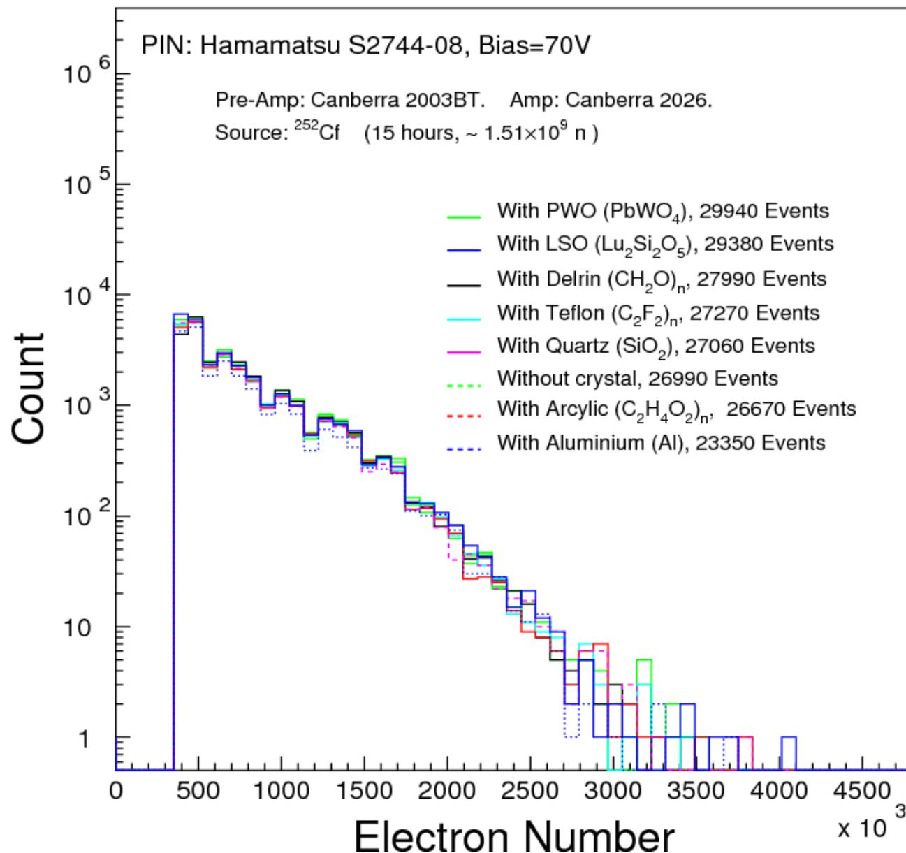
1 to 2 cm thick materials were inserted at the front of the PIN.
