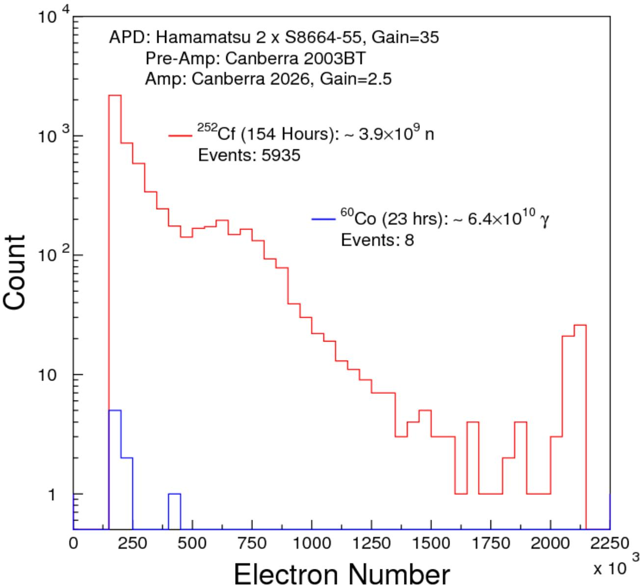
The trigger rate of MeV  $\gamma$ -rays from an  $^{60}\text{Co}$  source is 4 orders of the magnitude smaller than  $^{252}\text{Cf}$  neutrons, indicating that the contamination from  $\gamma$ -rays is negligible.
