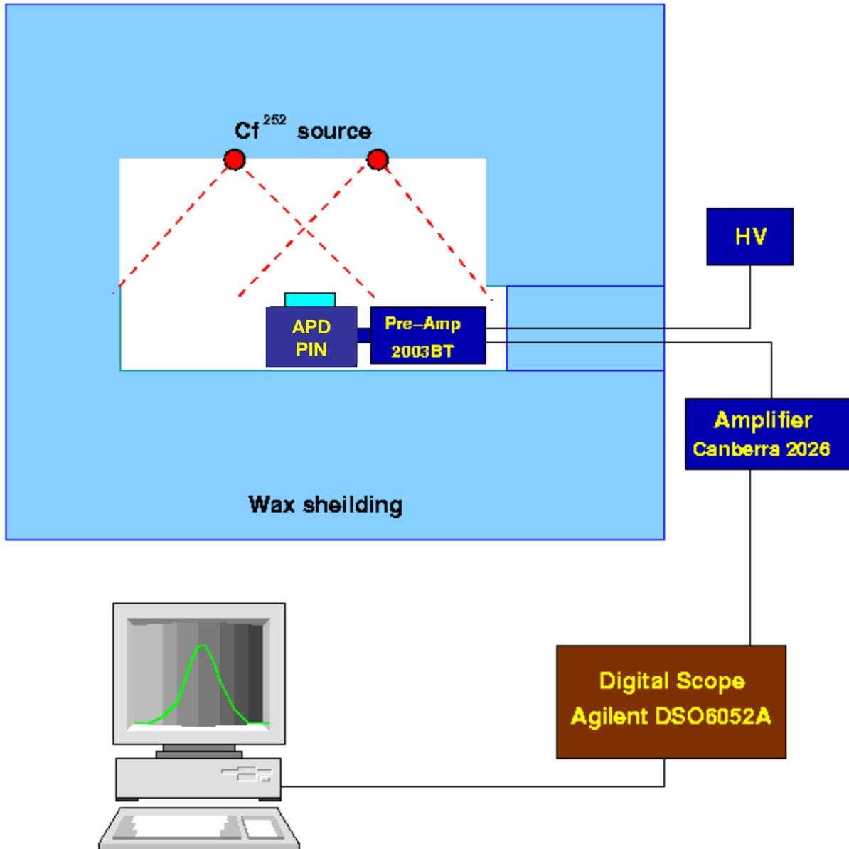
Si APDs/PIN were placed at 8 cm from a pair of  $^{252}\text{Cf}$  sources with neutron flux of  $1.4 \times 10^4$  n/cm<sup>2</sup>/s at the device surface.
