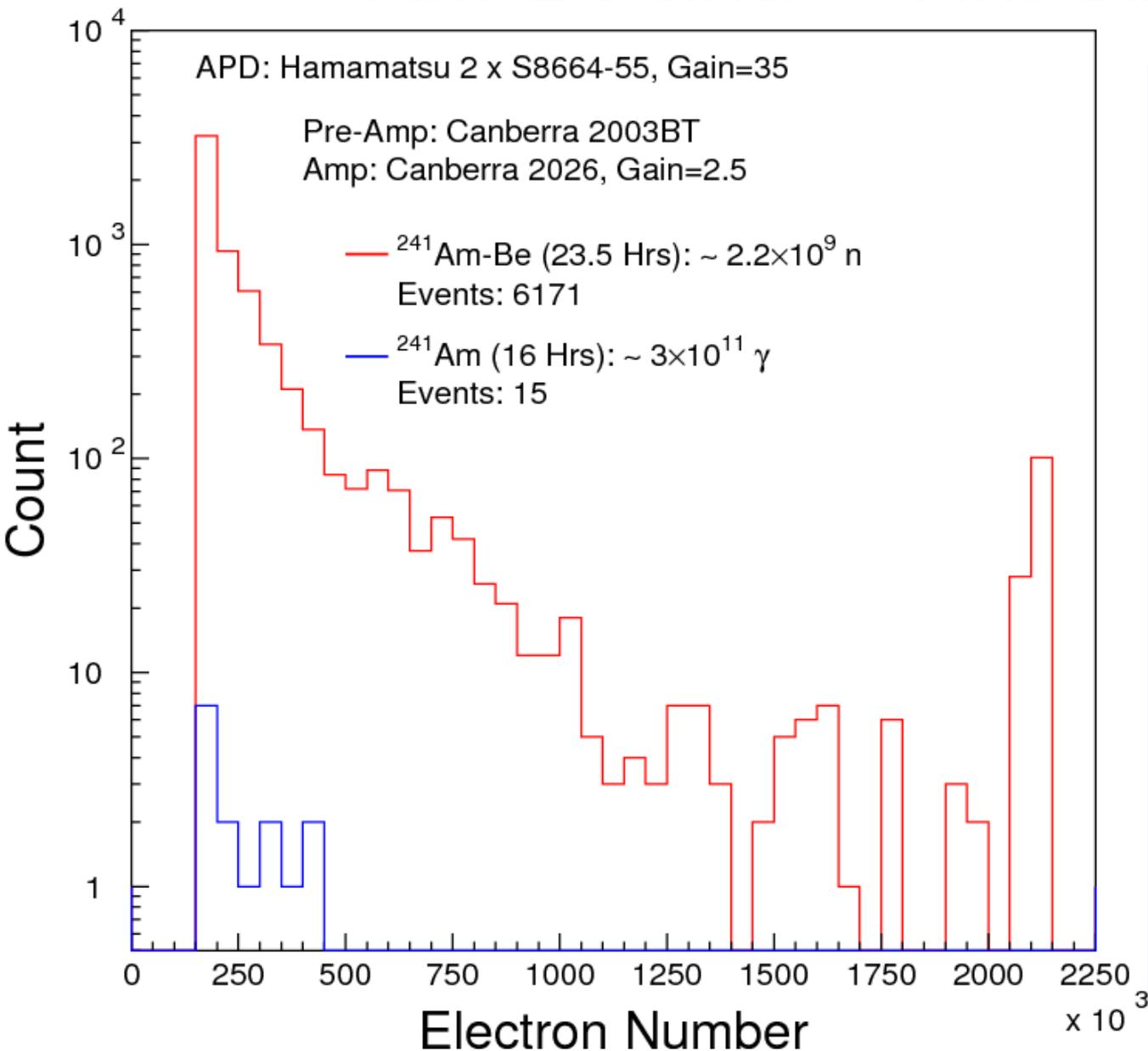
The trigger rate of 15 and 60 keV X-rays from an  $^{241}\text{Am}$  source is five orders of the magnitude smaller compared to  $^{241}\text{Am-Be}$  neutrons, indicating negligible contamination from X-rays.
