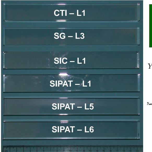
25 x 25 x 200 mm samples measured for their L.R.U. and fit to a linear function
