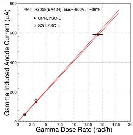
$\gamma$ -ray induced PMT anode current can be converted to the photoelectron numbers (Q) integrated in 100 ns gate. Its statistical fluctuation contributes to the readout noise ( $\sigma$ ): 0.2 & 1 MeV @ 15 & 500 rad/h.
