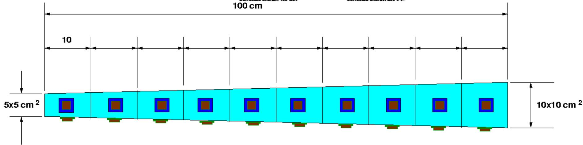
R.-Y. Zhu, ILCWS-8, Chicago: a HHCAL cell with pointing geometry
