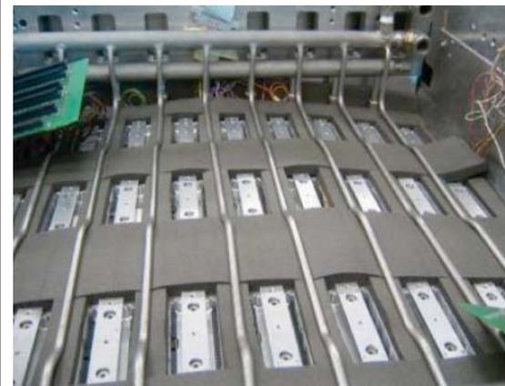
Water manifold and pipes on SM
