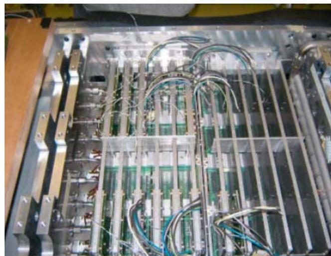
Cooling bars in direct contact with electronic cards
