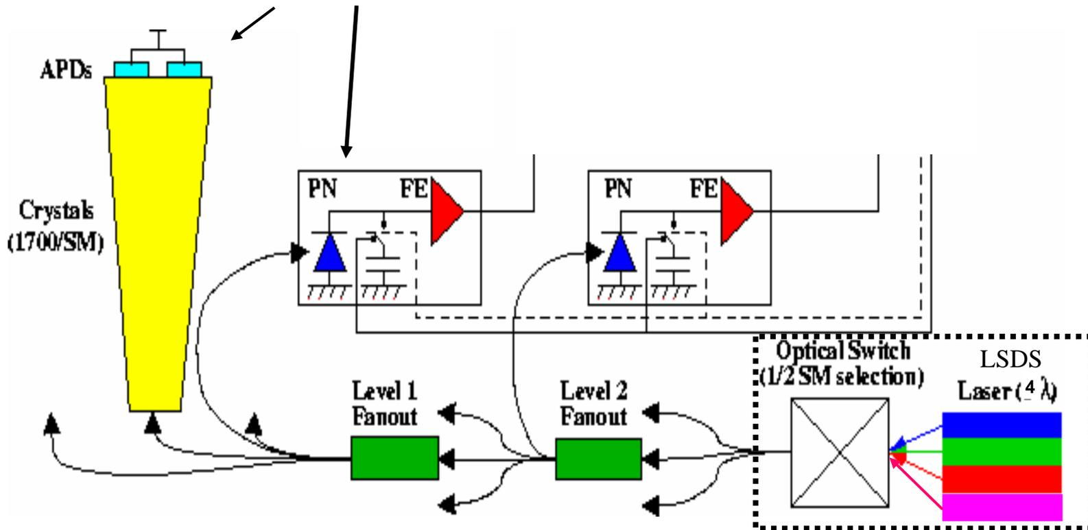
The ECAL light monitoring system consists of laser source, optical switch based high-level distribution system and two level fanout system.
