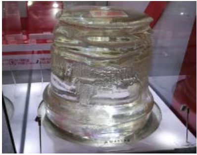
Large sapphire crystal of 400-450 kg
