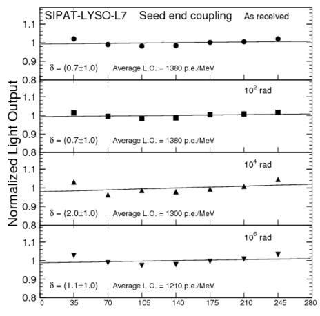
Distance from the end coupled to PMT (mm)
