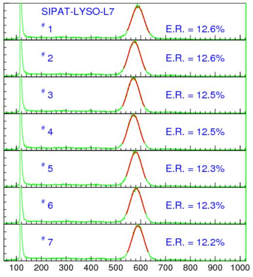
Corresponding FWHM energy resolution at seven points along the crystal was measured by using an R1306 PMT to be 12.4% in average.
