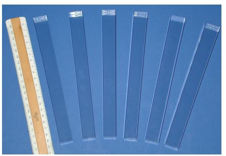
Sipat's Φ60 x 250 mm ingots are cut to two crystals for the SuperB beam test matrix. While crystals L11 to L16 are accepted, crystals L8, L9 & L10 were rejected because of poor optical transmittance.
