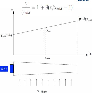
Light response uniformity at a few percents observed for both PMT and APD readouts.
