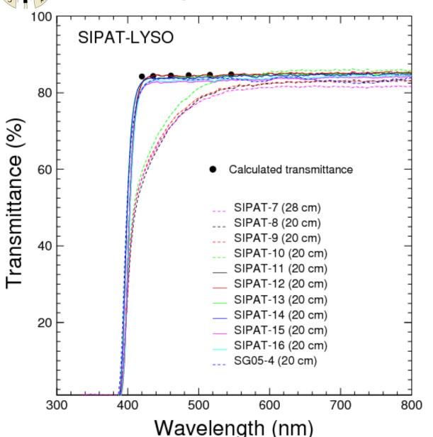
With rigorous control recently delivered LYSO crystals show no absorption band at the seed end.
