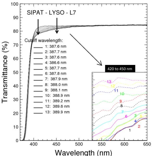
Poor transverse transmittance observed at the seed end of the crystal sample.
