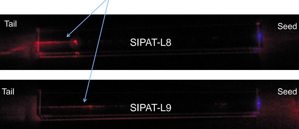
The low transmittance at the seed end is caused by absorption
