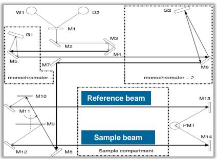
Perkin Elmer Lambda-950 spectrophotometer with double beam, double monochromator and GPOB for large samples.
