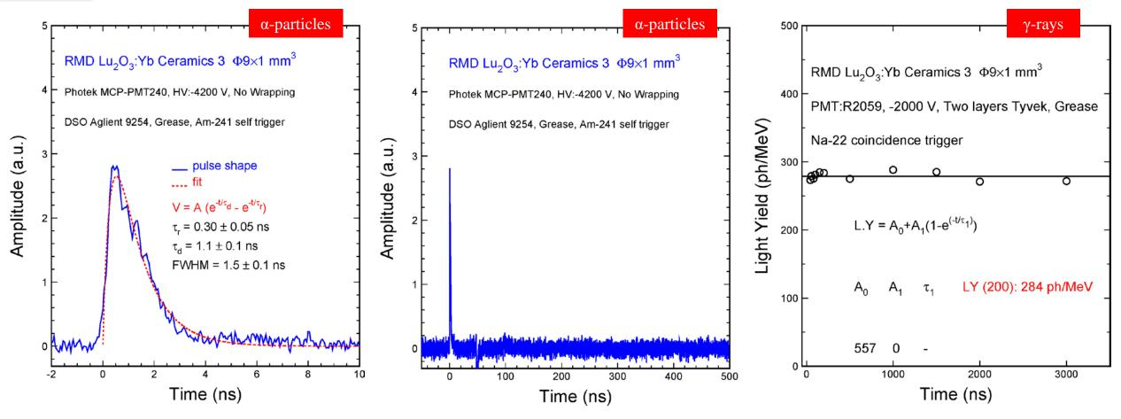
Lu<sub>2</sub>O<sub>3</sub>:Yb ceramic of 9.4 g/cc shows an ultrafast decay time of **1.1 ns** by Am-241 with negligible slow component observed in integrated light output measurement
