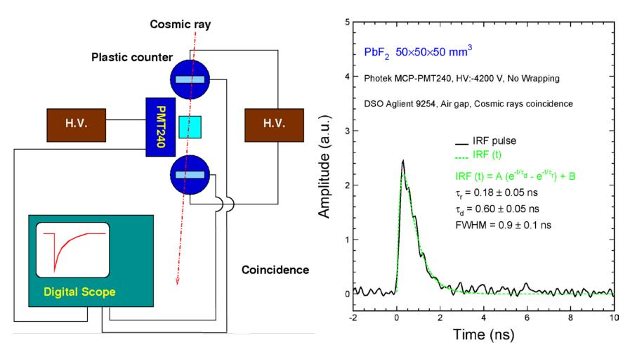
Intrinsic ultrafast response time can be extracted by taking out the IRF of the set-up. It was measured by fitting Cerenkov light pulse from a PbF<sub>2</sub> crystal, which agrees well with Photek spec.
