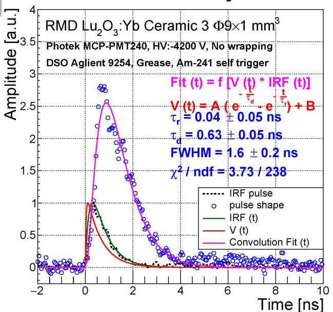
The magenta line shows the convolution fit. The numerical values of the fit after taking out the IRF are shown in blue
