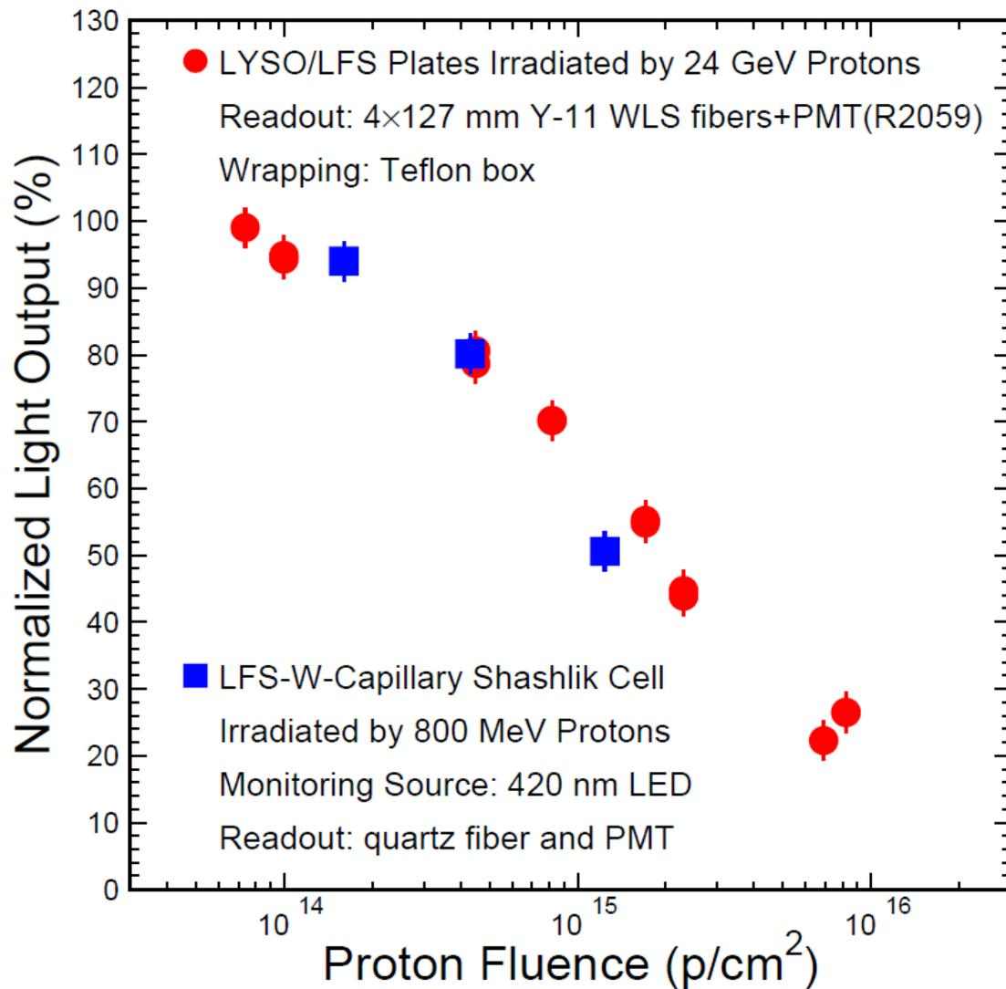
Consistent damage for plates and a Shashlik cell indicates small degradation in quartz capillaries & no difference between protons of 800 MeV and 24 GeV.
