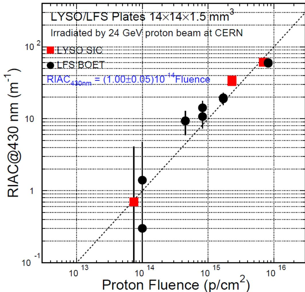
Consistent RIAC at 430 nm is observed in LYSO and LFS plates irradiated by 24 GeV protons up to  $8.19 \times 10^{15} \text{ p/cm}^2$  at CERN in 2014 and 2015.
