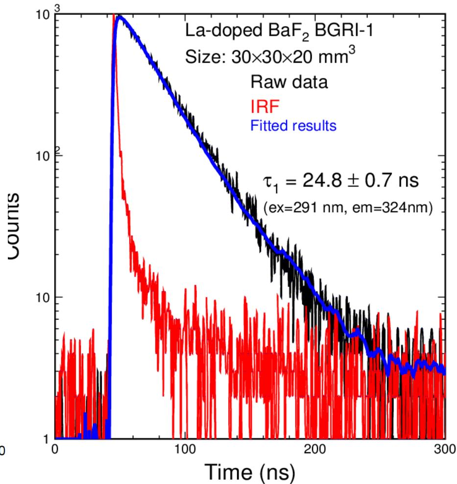
Decay kinetics was fit to three components to accommodate Ce emission
