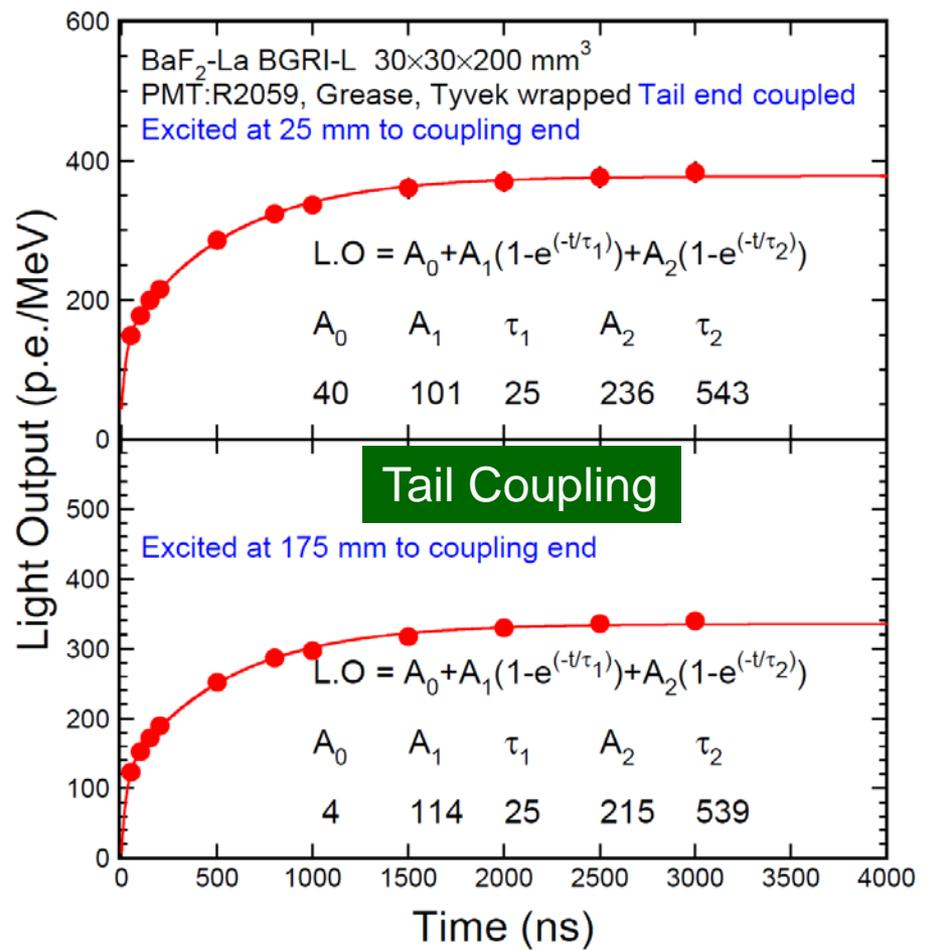
Consist F/S ratio after switching the coupling end
