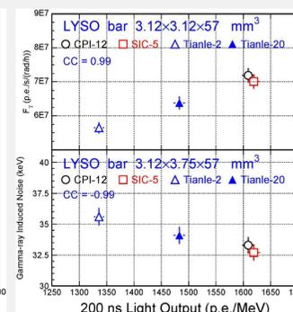
**Fig. 8** Correlation between F<sub>γ</sub> (top) and RIN: $\gamma$  (bottom) vs. LO in 200 ns gate for four LYSO+SiPM packages
