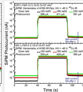
**Fig. 5** Histories of the SiPM photocurrent for CPI-12 (top) and SIC-5 (bottom) under Co-60 irradiation
