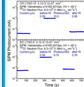
**Fig. 9** Histories of SiPM photocurrent for CPI-12 (top) and SIC-5 (bottom) before/during/after Cf-252 irradiation
