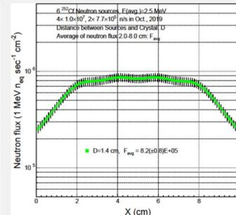
**Fig. 3** Neutron flux as a function of the position X in LYSO at D = 1.4 cm
