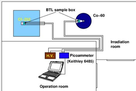
**Fig. 1** The setup used to measure photocurrent in LYSO+SiPM before, during and after irradiation
