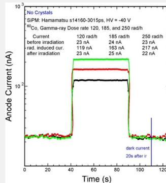
**Fig. 4** Histories of photocurrent measured for the SiPM under Co-60 irradiation
