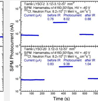
**Fig. 10** Histories of SiPM photocurrent for Tianle-2 (top) and Tianle-20 (bottom) before/during/after Cf-252 irradiation
