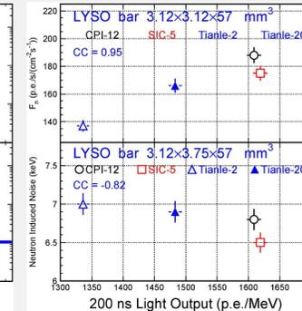
**Fig. 11** Correlation between F<sub>n</sub> (top) and RIN:n (bottom) vs. LO in 200 ns gate for four LYSO+SiPM packages
