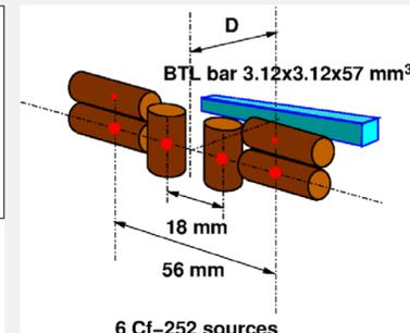
**Fig. 2** Three Cf-252 source pairs used as the neutron source group
