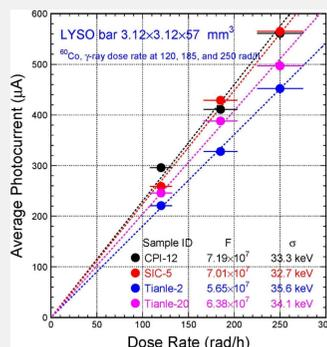
**Fig. 7** Photocurrent is shown as a function of the dose rate for four LYSO+SiPM packages
