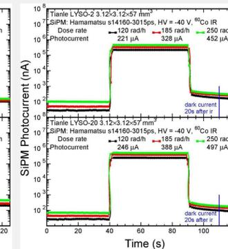
**Fig. 6** Histories of the SiPM photocurrent for Tianle-2 (top) and Tianle-20 (bottom) under Co-60 irradiation
