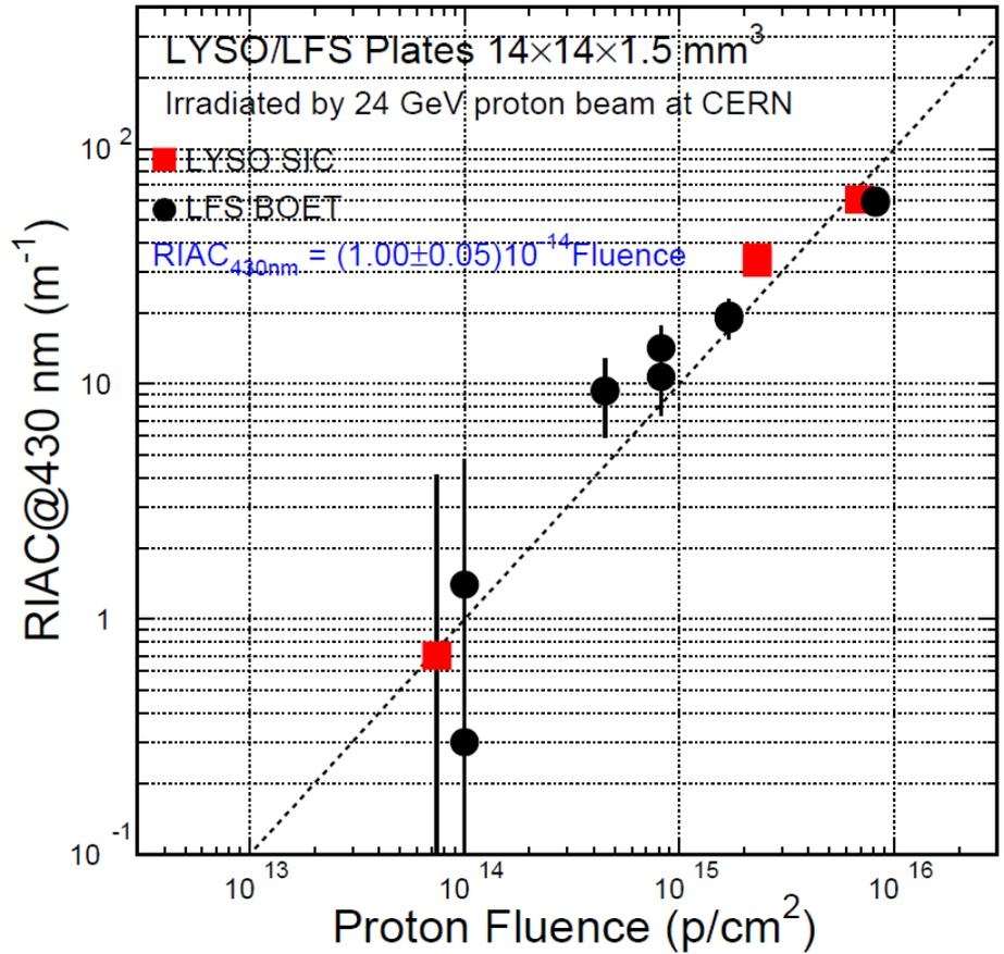
**Consistent damage in LFS and LYSO**
