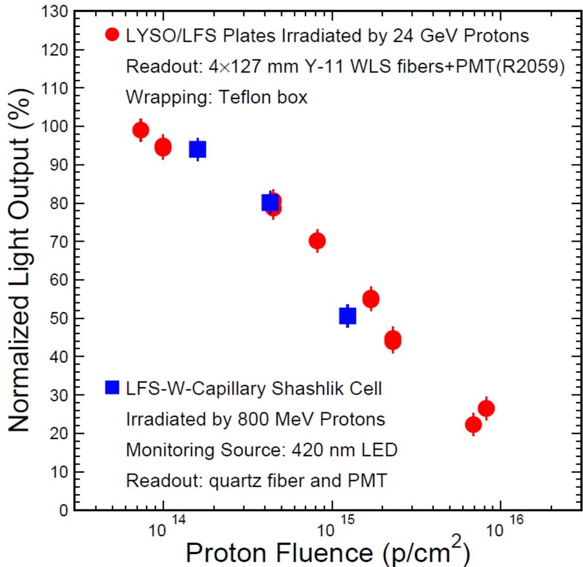
Consistent damage for plates and a Shashlik cell indicates small degradation in quartz capillaries & no difference between protons of 800 MeV and 24 GeV
