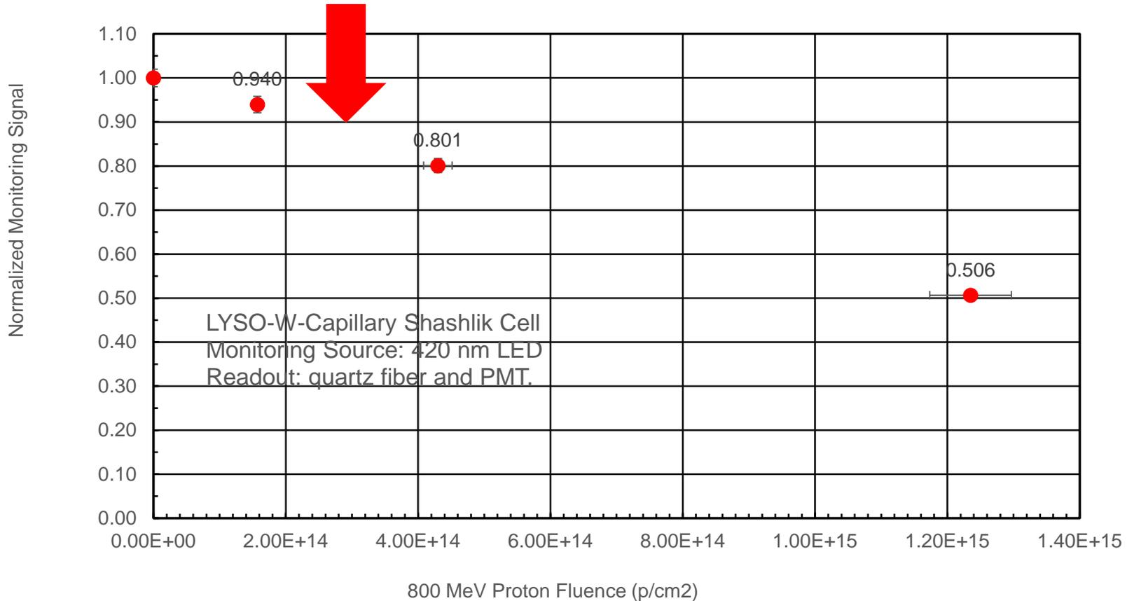
~10% light output loss in a LYSO/capillary based Shashlik tower
