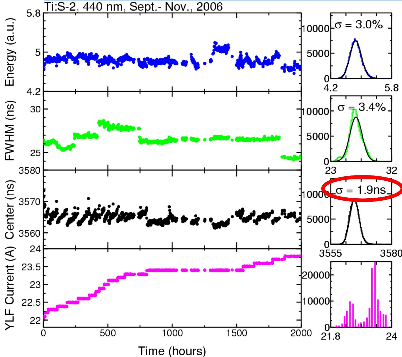
A factor of two better stability in laser pulse energy and width and a jitter of less than 2 ns were observed in laser runs lasting for about three months, when YLF current increased automatically at 0.1 nA steps.
