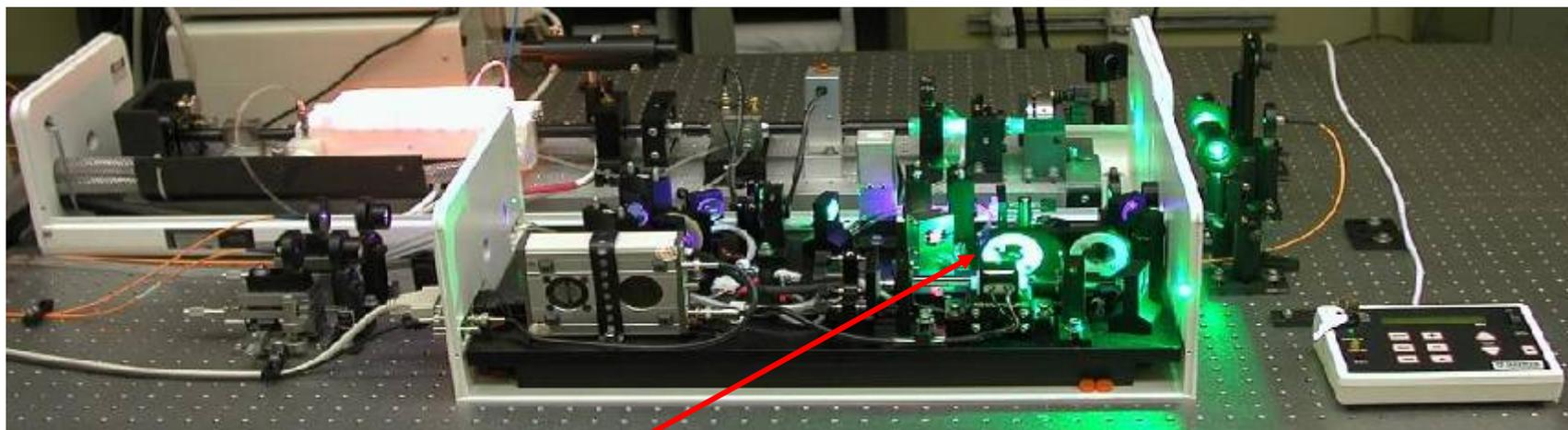
Lasers operate at two wavelengths by using interference filters in path
