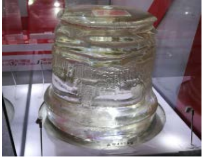
Large sapphire crystal of 400-450 kg
