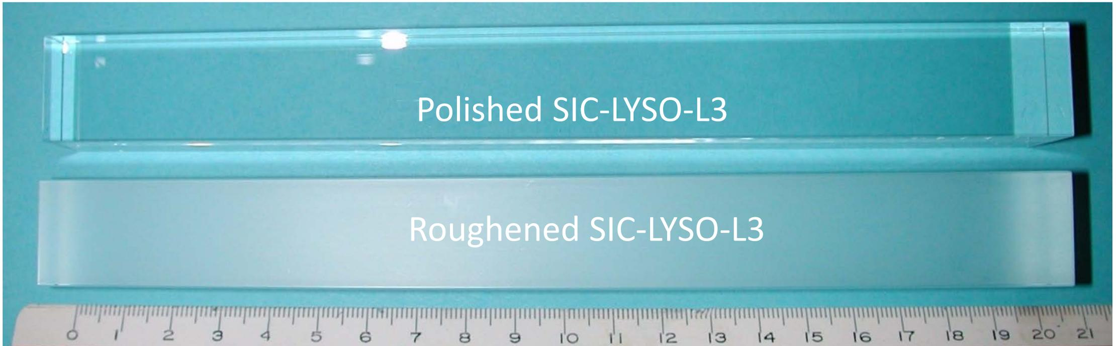
1st: lapped to  $R_a = 0.5$  by using  $11 \mu\text{m Al}_2\text{O}_3$  powder for 10 min with 2.5 kg weight
