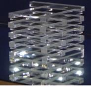
A LYSO matrix of 25 crystals was tested in May, 2011. Crystals were uniformized by black painting of 15 mm at the small end of the smallest side surface
