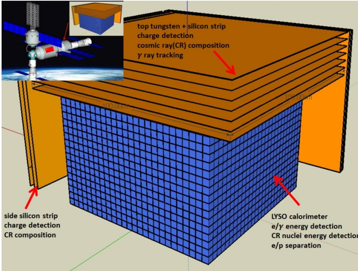
9261 LYSO crystals of 3 cm cube with WLF readout:
