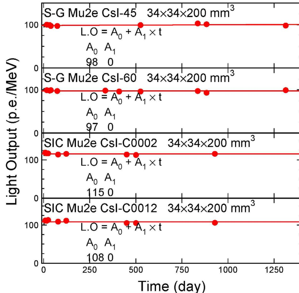
No recovery was observed up to 1,313 & 929 days for two CsI crystals each from SG and SIC respectively, indicating a stable calorimeter
