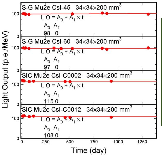
No recovery was observed up to 1,313 & 929 days for two Csl crystals each from S-G and SIC respectively, indicating a stable calorimeter
