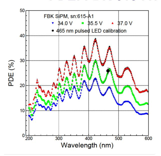
PDE scanned at 34.0, 35.5 and 37.0 V with gain measured.
