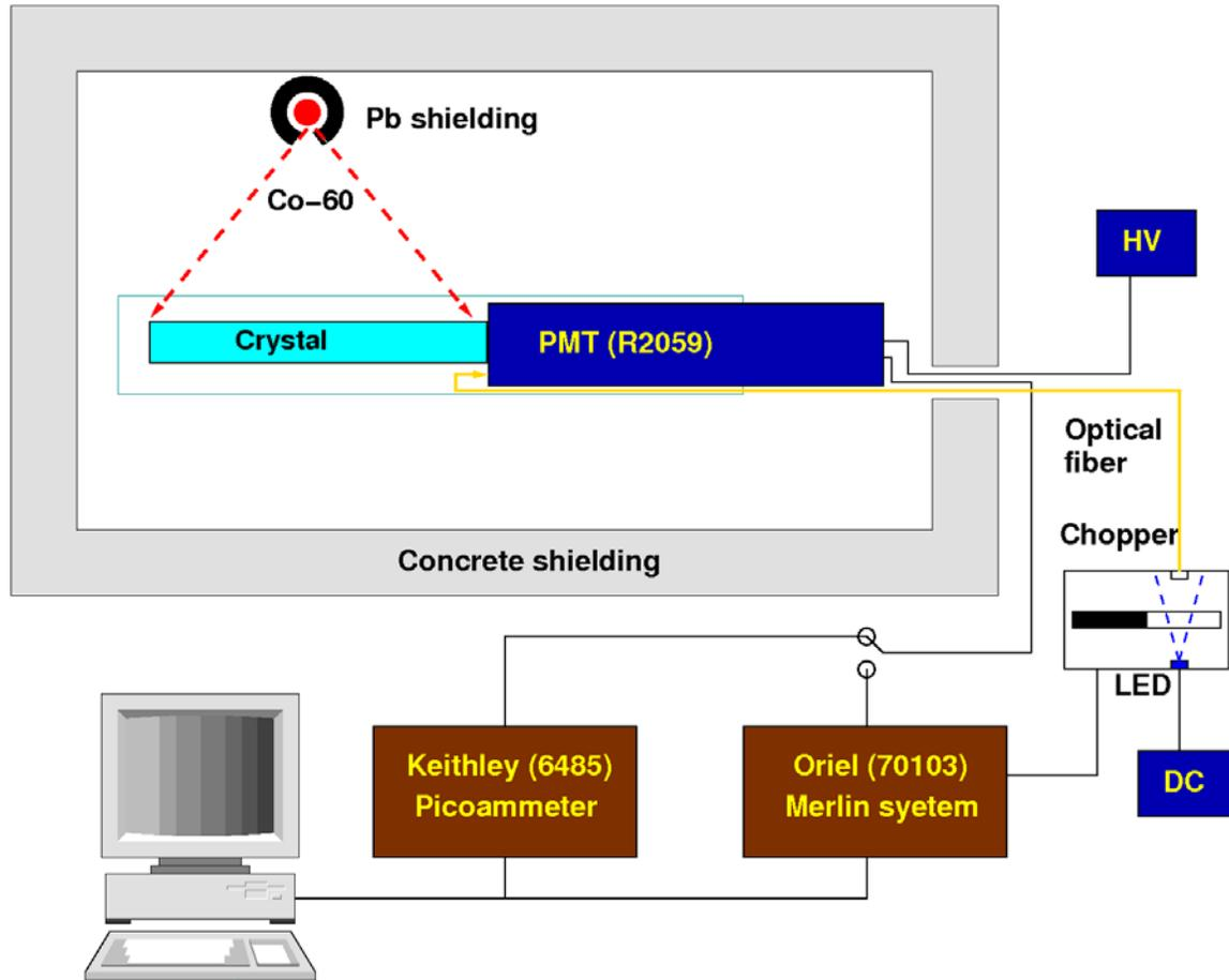
BaF<sub>2</sub> crystals, wrapped by Tyvek paper and coupled to the R2059 PMT via an air gap, were irradiated by <sup>60</sup>Co γ-rays under dose rates of 2 and 23 rad/h
