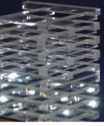
BaF<sub>2</sub> has a ultrafast scintillation component @ 220 nm with 0.5 ns decay time and an intensity similar to undoped CsI. It has also a factor of 5 larger slow component @ 300 nm with 300 ns decay time.
