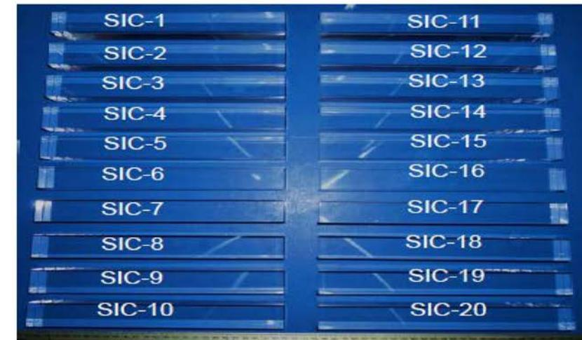
20 cm long BaF<sub>2</sub> shows ~50% light output loss after 120 Mrad, indicating good radiation resistance against ionization dose.
