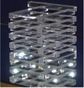
Average  $LO/\tau$  degrades by 8.9/17.1/17.8 % after  $\gamma/\gamma+n/\gamma+n+p$ , indicating a less than 5/10/10 % degradation in timing resolution
