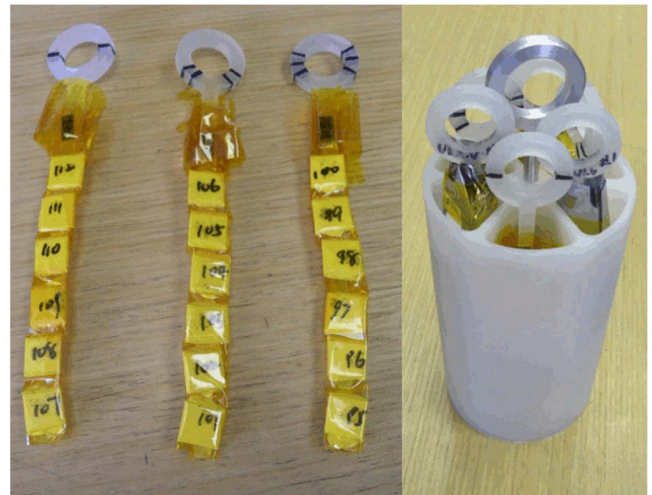
Fig. 3. Two photographs showing (left) three LFS plate bars and (right) sample holder hosting samples for experiment 6991.
