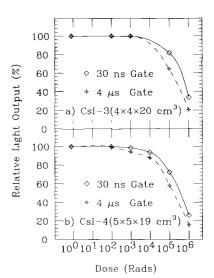
Fig. 5. Relative light yields measured with two different gate widths from two large size undoped CsI crystals are shown as a function of dosage.
