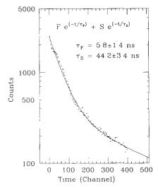
Fig. 2. Decay time spectrum (0.1 ns/channel) from an undoped CsI.
