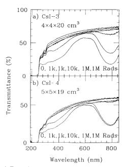
Fig. 4. Transmittance spectra of two large size undoped CsI crystals obtained before and after 100, 1 k, 10 k, 100 k and 1 Mrads of  $^{60}$ Co  $\gamma$ -ray irradiation.
