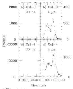
Fig. 3. <sup>137</sup>Cs pulse height spectra obtained from two large size undoped CsI crystals for two gate widths.
