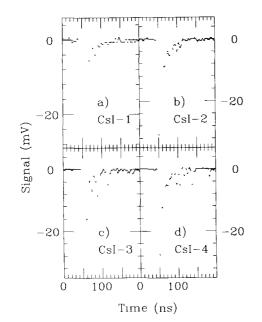
Fig. 1. Waveforms collected by a digital scope HD54111D from four undoped CsI samples: (a) CsI-1, (b) CsI-2, (c) CsI-3, (d) CsI-4.
