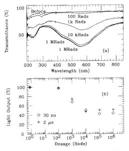
Fig. 6. Transmittance (a) and relative light output (b) measured with a 25 cm long  $BaF_2$  crystal from SIC are shown as a function of dosage.
