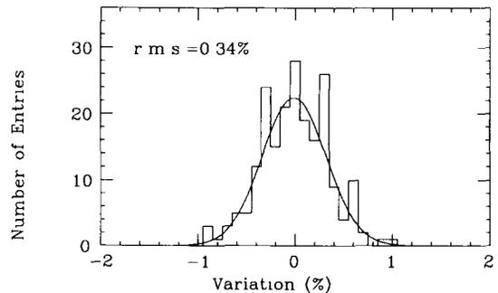
Fig. 7. Variation of the normalized peak positions from BGO crystals.
