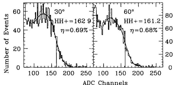
Fig. 3. A comparison of photon energy spectra of a BGO crystal with 5 MeV veto cut for two different incident angles:  $30^\circ$  and  $60^\circ$ .
