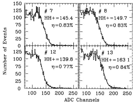
Fig. 2. Photon energy spectra and  $HH^+$  points for four BGO crystals without veto cuts.
