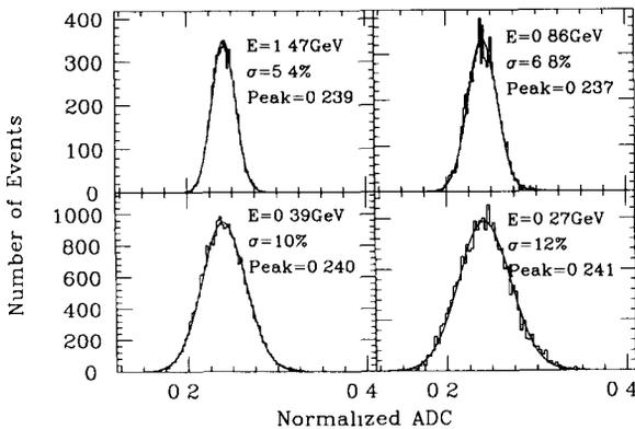
Fig. 5. Normalized ADC distribution of a crystal at different energies.
