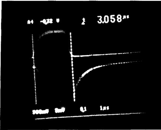
Fig. 4. RFQ beam pulse and the scintillation light pulse from a BaF<sub>2</sub> counter.
