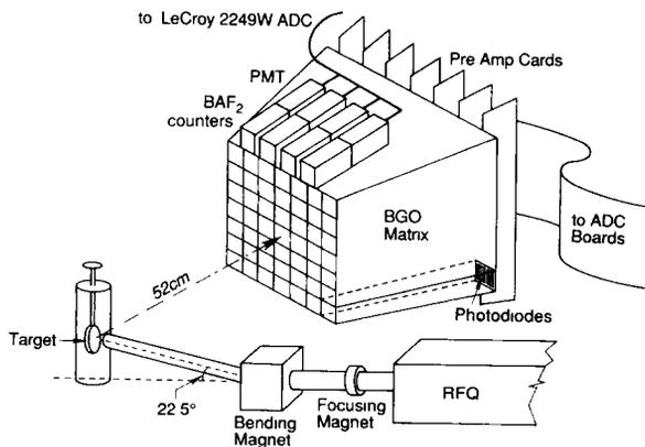
Fig. 1. AccSys test experimental setup.
