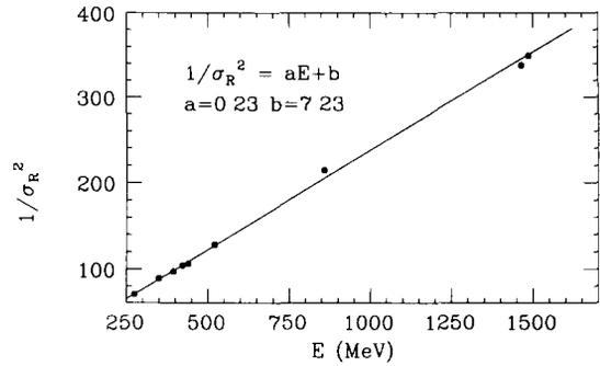
Fig. 6. Correlation between the relative rms and the average energy in a BGO crystal.
