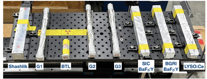
Fig. 2. Photograph showing eight samples mounted on the linear stage. Aluminum foils were taped to the two ends of G1, G2, G3, and BTL crystals and the front face of the Shashlik cell to measure proton fluence.
