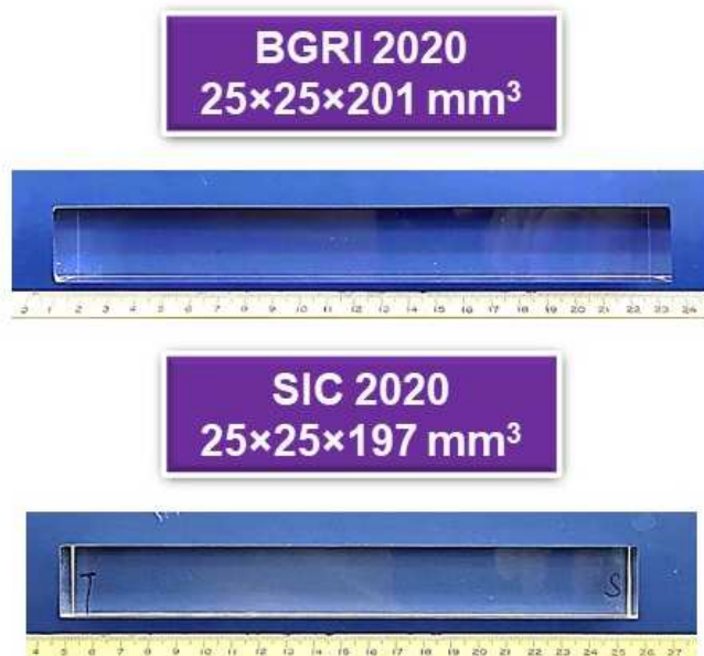
Fig. 1. Two BaF 2 :Y crystals grown by BGRI with a dimension of 25×25×201 mm 3 (top) and SIC with a dimension of 25×25×197 mm 3 (bottom) for the Mu2e-II experiment.
