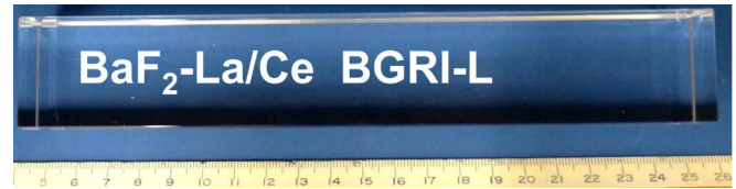
Fig. 12. 20-cm-long \text{BaF}_2 crystal co-doped with La and Ce.
