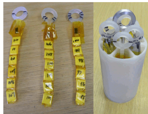
Figure 3 Three bars with LFS plates (Left) and the sample holder (Right) for the exp. 6991.
