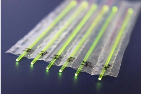
Fig. 10. YAG:Ce square fibers of 1 \times 1 \times 100 \text{ mm}^3 produced using fine cutting of large crystal by Crytur company.
