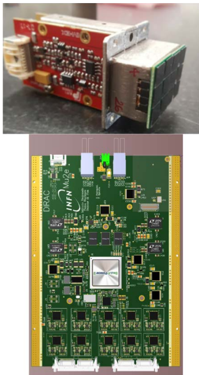
Fig. 11. Picture of the preproduction electronics: (top) example of two Amp-HV chips connected to the back of the Left and Right SiPM arrays on their holder; (bottom) the first version of the calorimeter digitizer (DIRAC).
