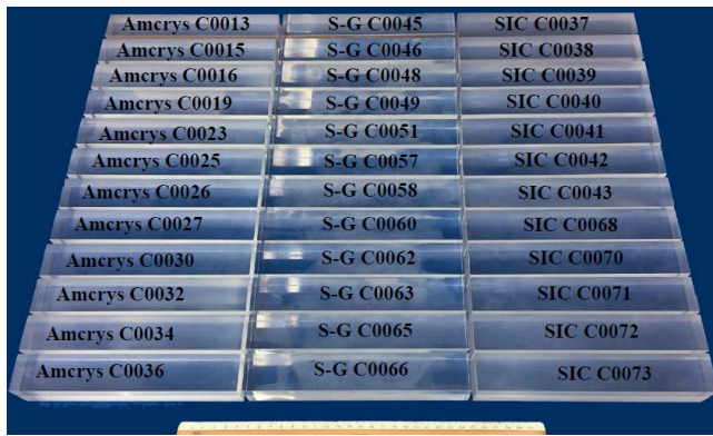
Fig. 1. 36 CsI crystals of 34 \times 34 \times 200 \text{ mm}^3 from Amcrlys, S-G, and SIC.
