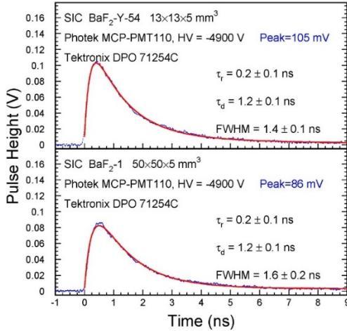
Fig. 3. Singlet bunch measured by  $\text{BaF}_2:\text{Y}$  (top) and  $\text{BaF}_2$  (bottom) coupled to the Photek MCP-PMT110.
