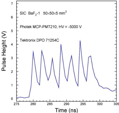
Fig. 4. Septuplet with 2.83 ns bunch spacing observed by  $\text{BaF}_2$  coupled to the Photek MCP-PMT 210.
