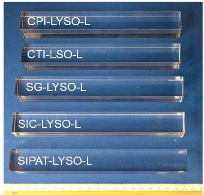
Fig. 1. A photo showing five LYSO crystals of 2.5 \times 20 \times 2.5 \text{ cm}^3 .
