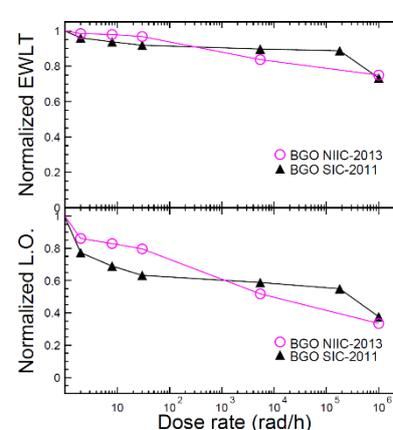
**Figure 6.** Normalized EWLT (top) and LO (bottom) are shown as a function of dose rate for two BGO crystals from different vendors.
