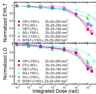
**Figure 1.** Normalized EWL and LO are shown as a function of integrated dose up to 340 Mrad for six LYSO/LSO/LFS crystals from different vendors.
