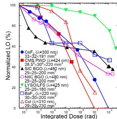
**Figure 9.** Normalized LO as a function of integrated dose for various crystals
