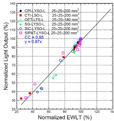
**Figure 2.** Correlation between normalized EWL and LO is shown for six LYSO/LSO/LFS crystals from different vendors.
