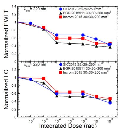
**Figure 4.** Normalized EWLT and LO of the fast scintillation component as a function of integrated dose for three BaF<sub>2</sub> crystals from different vendors.
