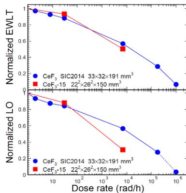
**Figure 7.** Normalized EWL T (top) and LO (bottom) are shown as a function of dose rate for two CeF<sub>3</sub> crystals
