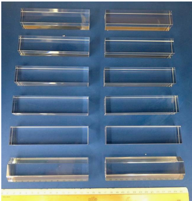
Fig. 2. Twelve 13 cm long LYSO crystals for Mu2e.
