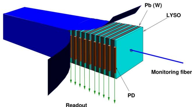
Fig. 11. Conceptual design of an LYSO-Pb sampling calorimeter cell readout by photo-detectors directly coupled to the edges of the crystal plates.
