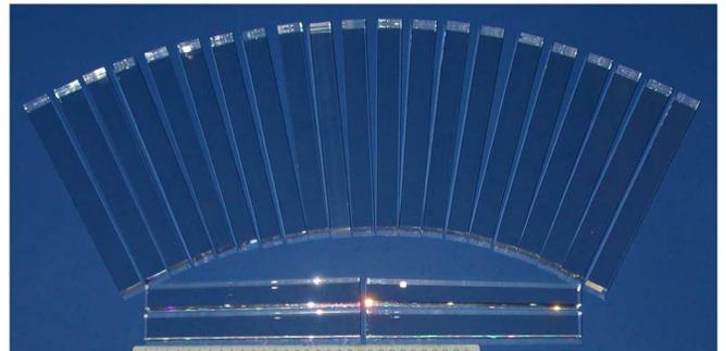
Fig. 1. Twenty five LYSO crystals with tapered geometry.
