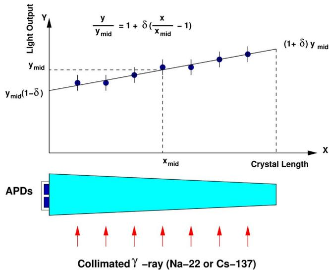
Fig. 2. Schematic showing the light response uniformity measurement.
