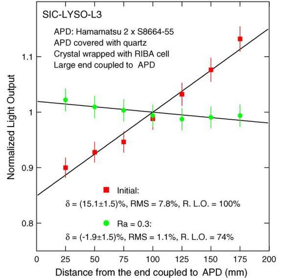
Fig. 8. Light output is shown as a function of the distance to the photo-detector for a tapered LYSO crystal before and after roughening the smallest side surface to  $R_a = 0.3$ .
