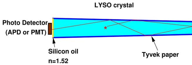
Fig. 6. Set-up used for the ray-tracing simulation described in the text.
