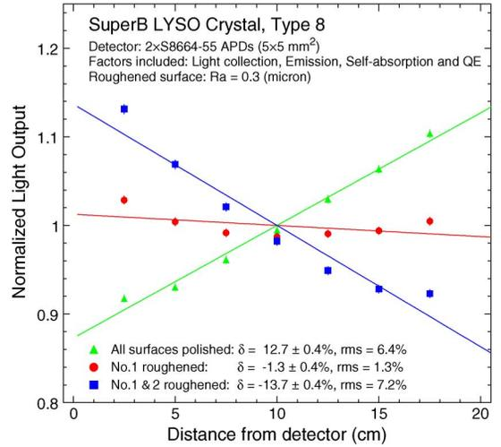
Fig. 7. Light output of a SuperB type 8 crystal is shown as a function of the distance to the photo-detector with (1) all surfaces polished; (2) one surface roughened to  $R_a = 0.3$  and (3) two surfaces roughened to  $R_a = 0.3$ .
