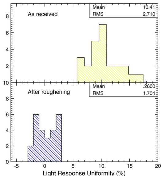
Fig. 9. LRU Summary of 25 SuperB LYSO crystals before and after one-surface roughening uniformization.
