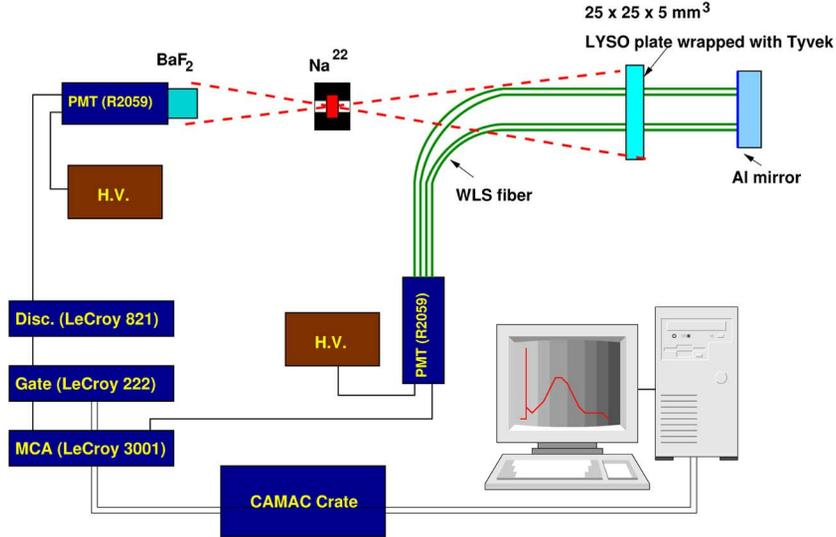
Fig. 12. Schematic showing the setup used to measure the light output of LYSO plates through four Y-11 WLS fibers.
