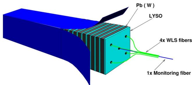
Fig. 10. Conceptual design of an LYSO-Pb Shashlik sampling calorimeter cell readout by WLS fibers.
