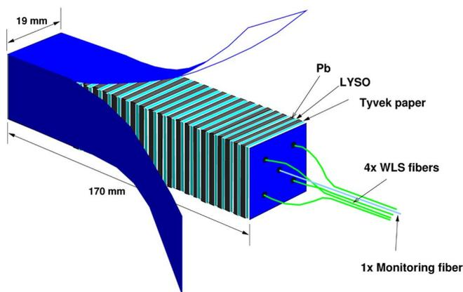
Fig. 16. Conceptual design of an LYSO crystal based Shashlik ECAL cell with lead as absorber and four Y-11 WLS fibers readout for a beam test.
