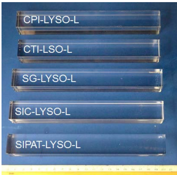
Figure 1. Five 20 \times 20 \times 200 mm 3 LSO/LYSO crystals from CPI, CTI, SG, SIC and SIPAT.
