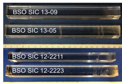
**Figure 2.** Four 20 cm long BSO crystal samples grown at SIC
