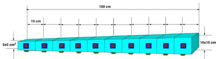
**Figure 1.** A schematic showing a typical cell for the HHCAL detector concept
