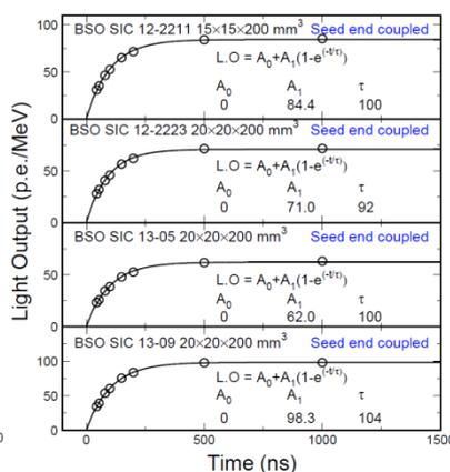
**Figure 4.** Initial Decay kinetics of four BSO samples
