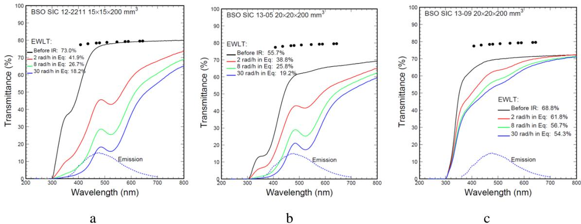
**Figure 6.** LT of three BSO samples in equilibrium under dose rates of 2, 8 and 30 rad/h: a. SIC 12-2211; b. SIC 13-05; and c. SIC 13-09.
