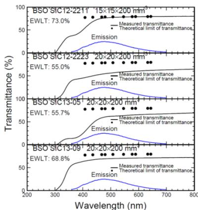
**Figure 3.** Initial LT of four BSO samples
