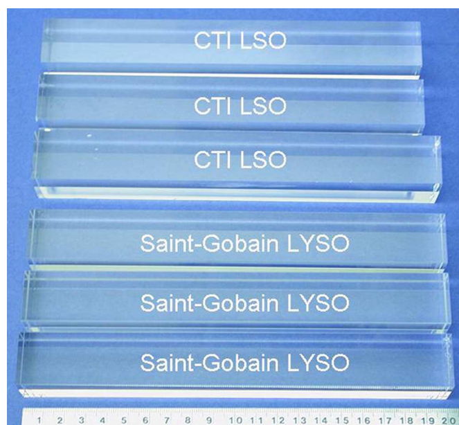
Fig. 2. Photo showing six LSO/LYSO crystal samples used in this study.
