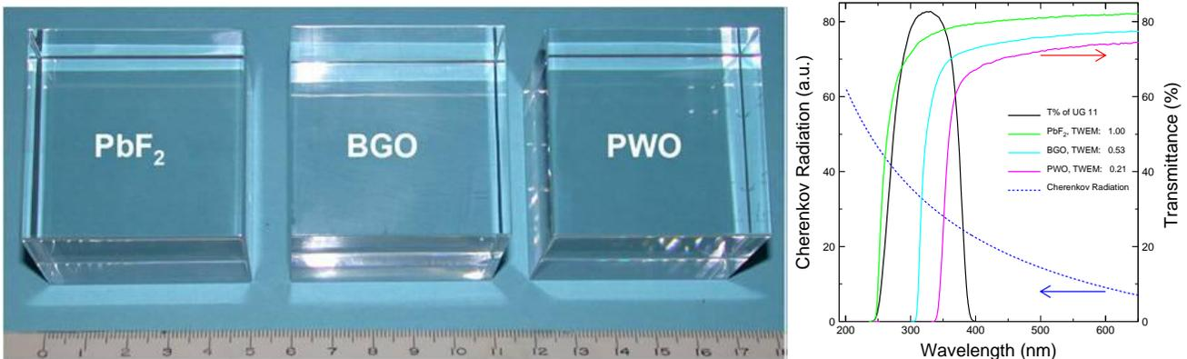
Figure 17. Left: A photo shows three crystal samples of  $5 \times 5 \times 5 \text{ cm}^3$  investigated for the homogeneous hadronic calorimeter concept. Right: The transmittance spectra of PbF<sub>2</sub> (green), BGO (blue), PWO (red) and UG 11 (black) are shown as a function of wavelength. Also shown in this figure are the Cherenkov emission spectrum (dashed blue) and the normalized figure of merit for the Cherenkov light measurement with the UG 11 filter.
