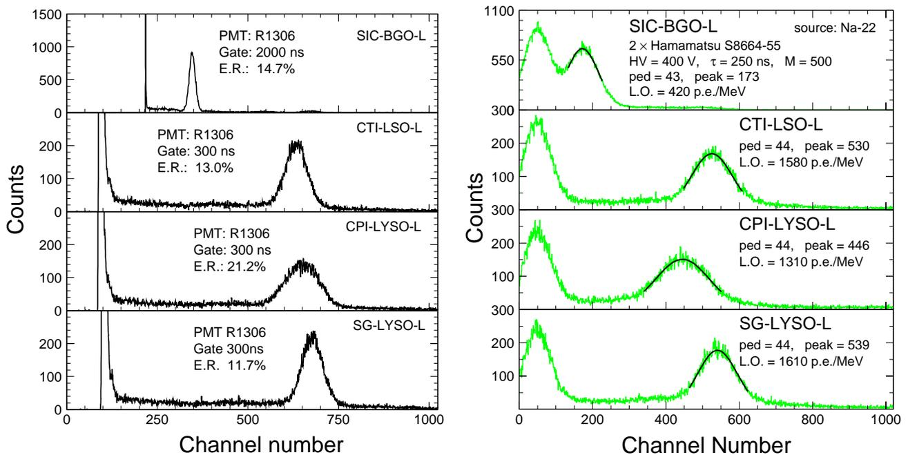
Figure 11. The spectra of  $0.511 \text{ MeV}$   $\gamma$ -rays from a  $^{22}\text{Na}$  source measured with a coincidence trigger using a Hamamatsu R1306 PMT (Left) and two Hamamatsu S8664-55 APDs (Right) for long BGO, LSO and LYSO samples of  $2.5 \times 2.5 \times 20 \text{ cm}^3$  size.
