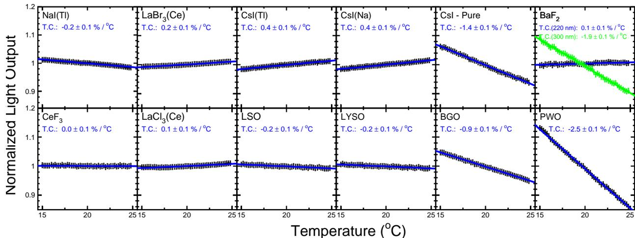
Figure 9. Light output temperature coefficient obtained from linear fits between 15°C and 25°C for twelve crystal scintillators.
