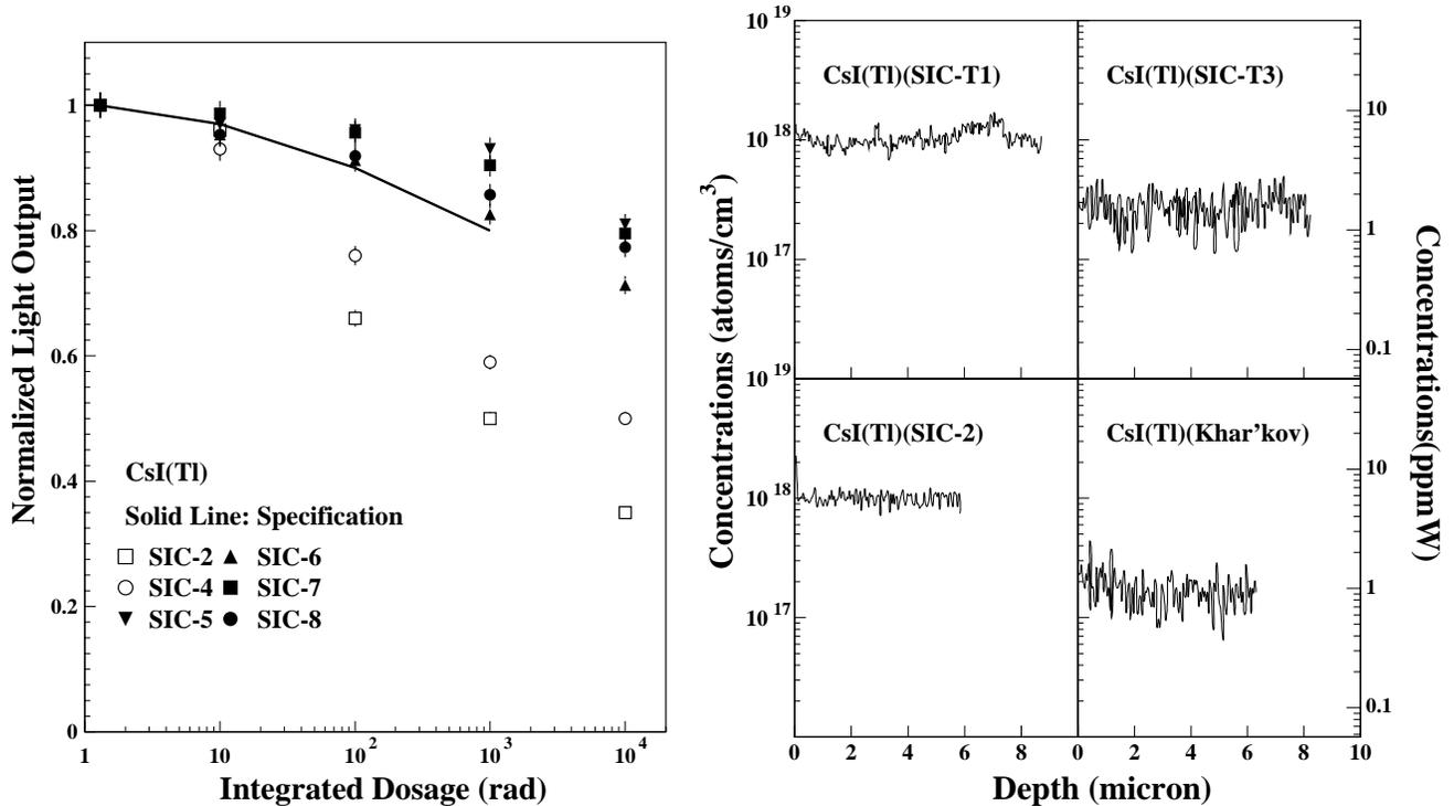
Figure 15. Left: The progress of CsI(Tl) radiation hardness is shown for full size ( $\sim 30$  cm) CsI(Tl) samples from SIC together with the rad-hard specification of the *BaBar* experiment. Right: The depth profile of oxygen contamination is shown for two rad-soft CsI(Tl) samples (SIC-T1 and SIC-2) and two rad-hard samples (SIC-T3 and Khar'kov).
