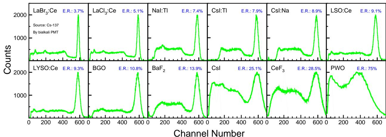
Figure 6. <sup>137</sup>Cs  $\gamma$ -ray pulse height spectra measured by a Hamamatsu R1306 PMT for twelve crystal samples with numerical values of the FWHM resolution (E.R.) also shown in the figure.
