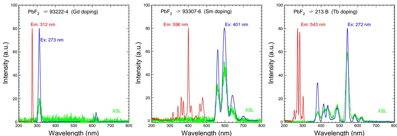
Figure 18. UV excitation (red), photo-luminescence (blue) and x-luminescence (green) spectra are shown as a function of wavelength for Gd (Left), Sm (Middle) and Tb (Right) doped  $\text{PbF}_2$  samples.
