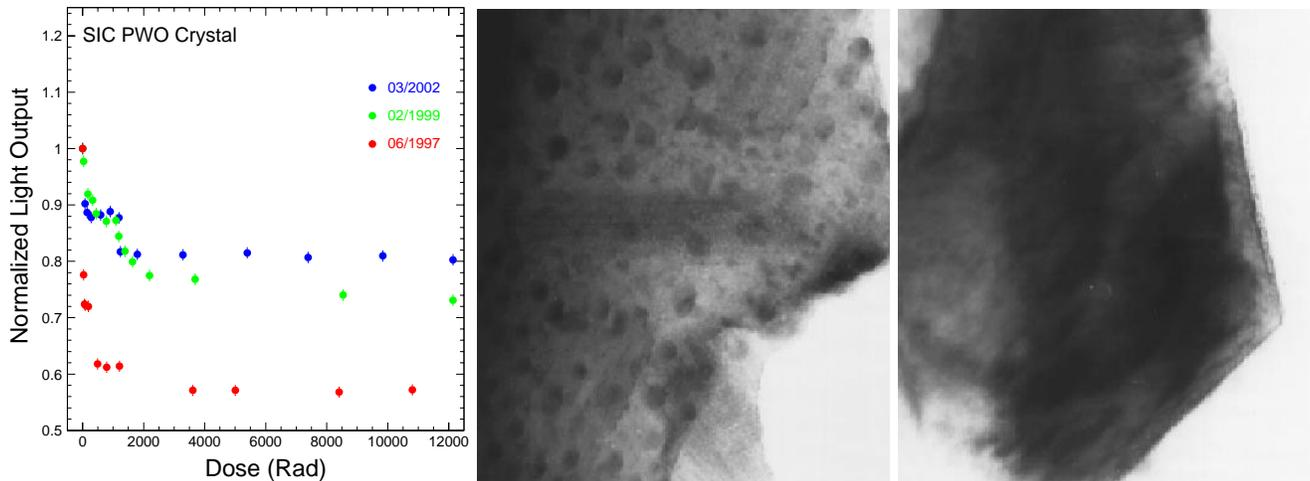
Figure 16. Left: The progress of  $\text{PbWO}_4$  radiation hardness is shown for full size (23 cm) CMS  $\text{PbWO}_4$  samples from SIC. TEM pictures of a  $\text{PbWO}_4$  crystal of poor (Middle) radiation hardness, showing clearly the black spots of  $\phi 5\text{--}10$  nm related to oxygen vacancies, as compared to that of a good one (Right)
