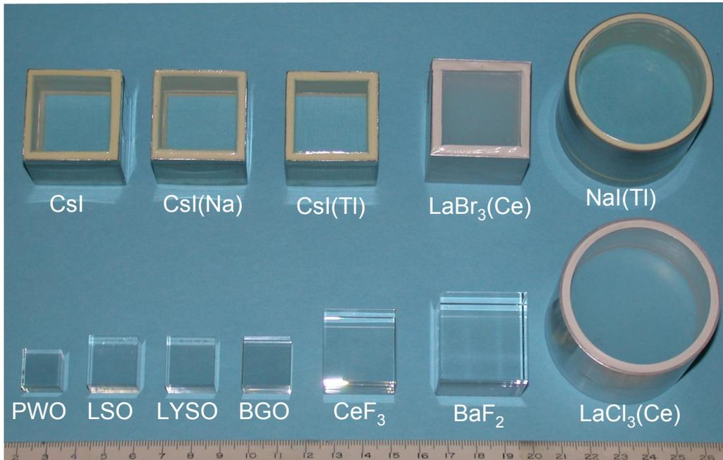
Figure 4. A photo shows twelve crystal scintillators with dimension of 1.5 X<sub>0</sub>.
