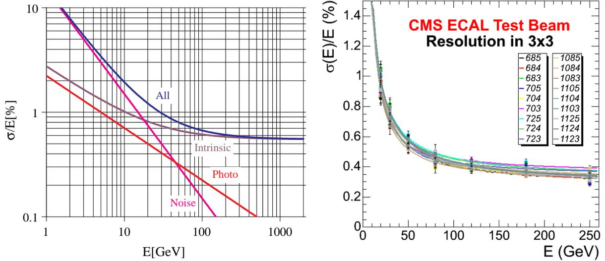
Figure 3. Left: The designed energy resolution of the CMS PbWO<sub>4</sub> calorimeter and corresponding contributions is shown as a function of energy.<sup>3</sup> Right: The energy resolution of two groups of 9 PbWO<sub>4</sub> crystals is shown as function of electron energy obtained in the CMS ECAL beam test.<sup>6</sup>
