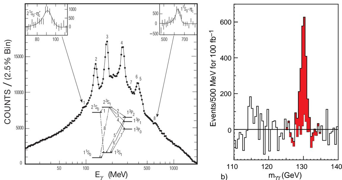
Figure 1. Left: An inclusive photon spectrum measured at the  $\psi'$  by the NaI(Tl) crystal calorimeter of the Crystal Ball experiment at SLAC.<sup>2</sup> Right: The expected background subtracted Higgs mass peak reconstructed from its two photon decays measured by the CMS PbWO<sub>4</sub> crystal calorimeter.<sup>3</sup>
