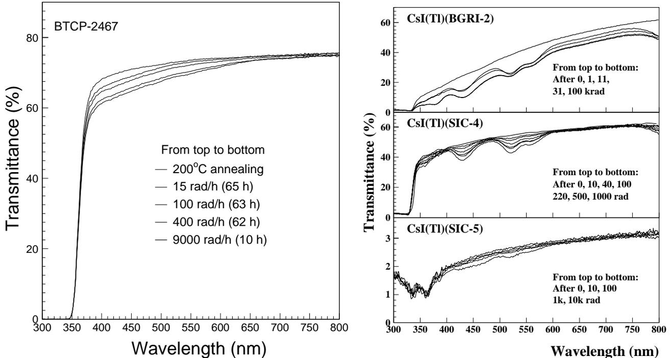
Figure 12. Longitudinal transmittance of  $\text{PbWO}_4$  (Left) and CsI(Tl) (Right) samples, showing radiation induced absorption bands.
