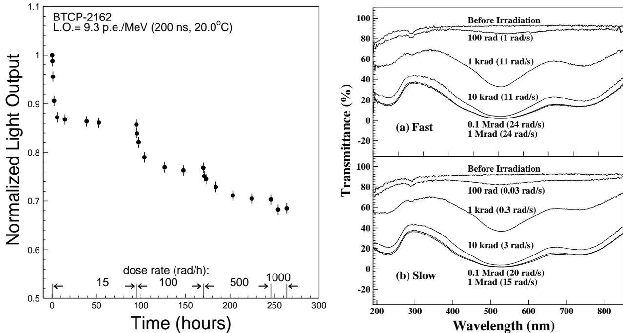
Figure 13. Left: Normalized light output is plotted as a function of time under irradiation for a CMS  $\text{PbWO}_4$  sample, showing dose rate dependent radiation damage. Right: No dose rate dependence was observed for the longitudinal transmittance spectra measured for a GEM full size  $\text{BaF}_2$  sample.
