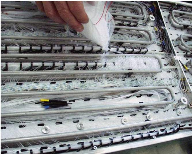
Fig. 17. Molded polyethylene grains, used as a neutron moderator, are filled into the region occupied by the monitoring system before the front cover of the SM is mounted.
