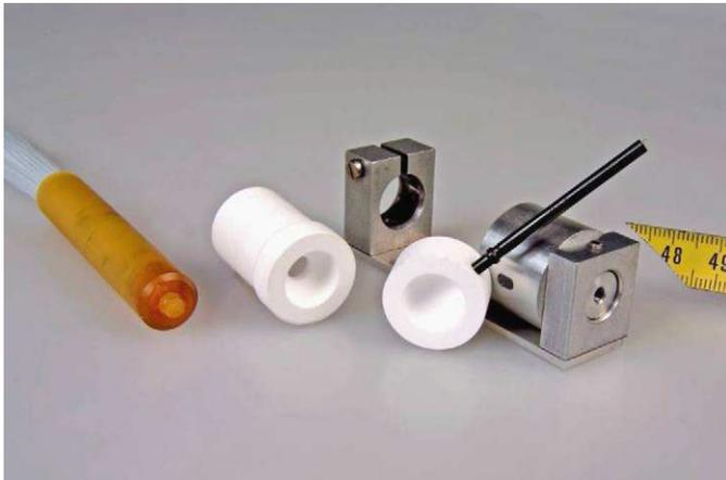
Fig. 9. ECAL barrel tertiary (L1) 240-fiber optical fan-out assembly. The fan-out inserts into a 12 mm ID diffusing sphere (shown opened here). Light is injected at 90° to the fan-out's axis via the ferrule.
