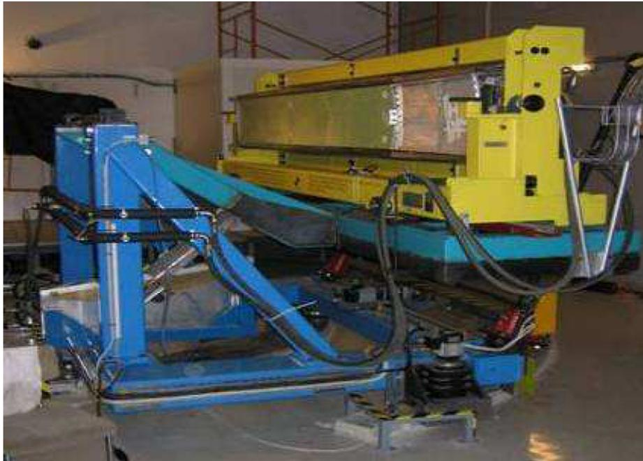
Fig. 32. SM mounted on automated scanning table in CERN H4 electron test beam.
