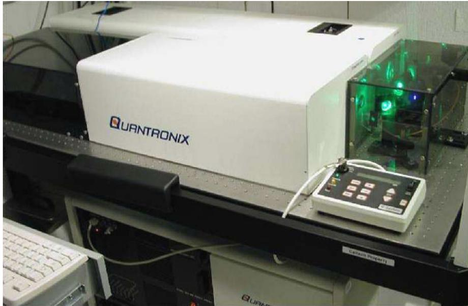
Fig. 3. Monitoring system multiple wavelength light source (shown installed at CERN H4 test-beam area).
