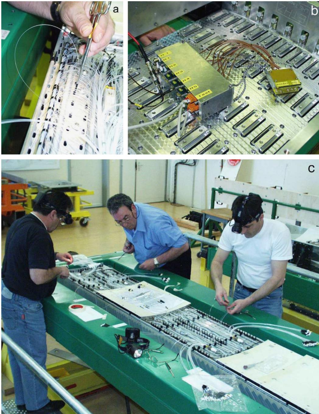
Fig. 29. Installation of the monitoring distribution system on an ECAL barrel SM: (a) shows tool used to insert the optical fiber's ferrule into a crystal's ferrule support, (b) shows the 10-channel amplifier and connector used to test APD response after cabling (SM face down), and (c) shows the installation of optical fibers on alternate sub-modules (SM rotated, front face up).
