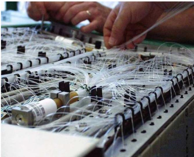
Fig. 10. ECAL barrel tertiary (L1) fan-out and its diffusing sphere assembly shown installed on a SM front face.
