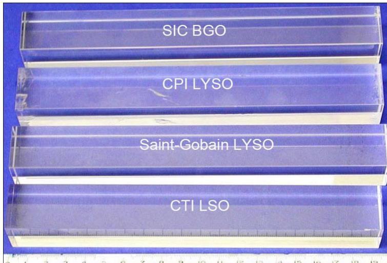
**FIGURE 8.** A photo shows four long crystal samples with dimension of  $2.5 \times 2.5 \times 20$  cm<sup>3</sup>.
