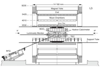
Fig. 3. Installation of the RFQ calibration system in the L3 detector at LEP [7].
