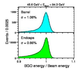
Fig. 4. Normalized Bhabha electron energy spectra measured by L3 BGO crystal calorimeter at LEP by using RFQ calibration.
