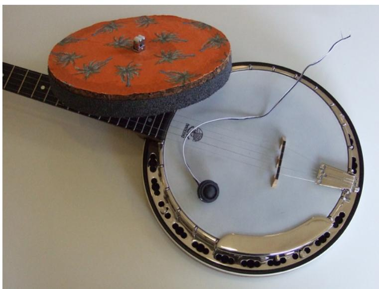
FIG. 1. Resonator banjo, 3/4" tweeter, and synthetic belly
