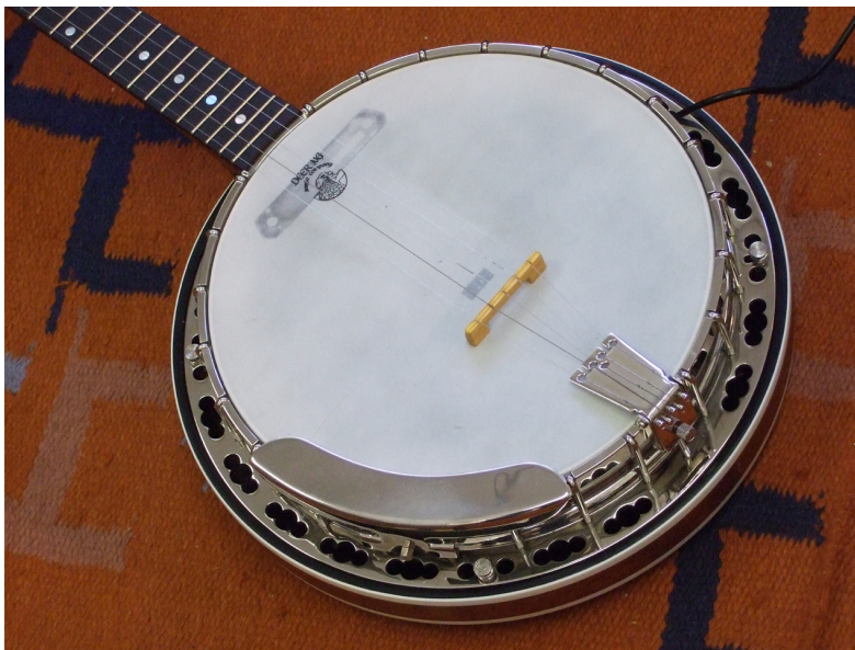
FIG. 1. something to try: a rare-earth sound hole pickup double-sticky-taped inside the head, as close to the rim as possible, with a lighter than “normal” bridge (e.g., 1.7 instead of 2.6 gm). Pickups mounted to the bottom of the head show through; paint it white before attaching, if you don’t want it to show as much.
