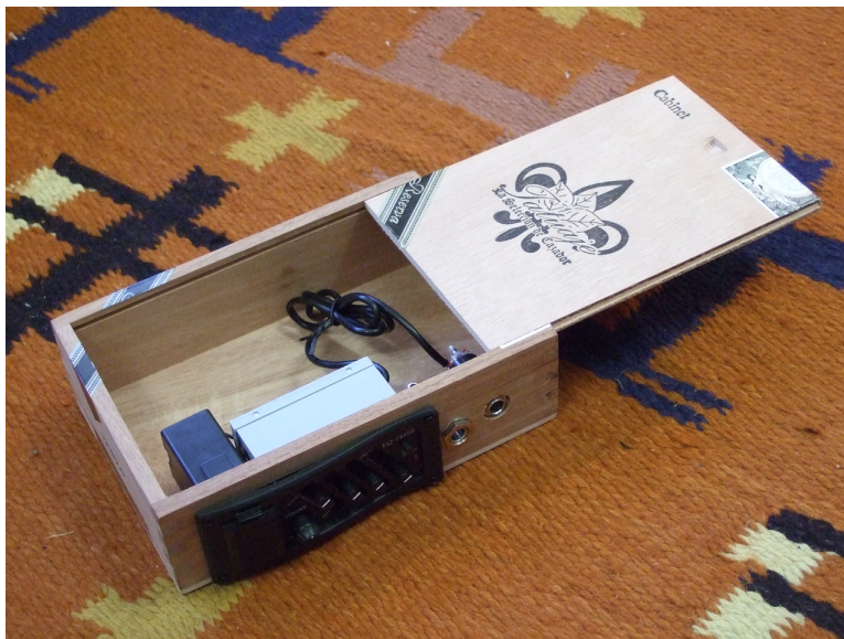
FIG. 3. an inexpensive ($8 if you're patient), op-amp based, commercial guitar pre-amp, with volume control and a four channel equalizer
