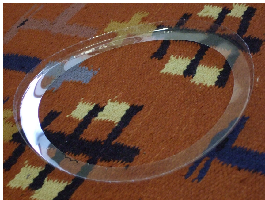
FIG. 4. Mylar ring cut from a clear mylar head
