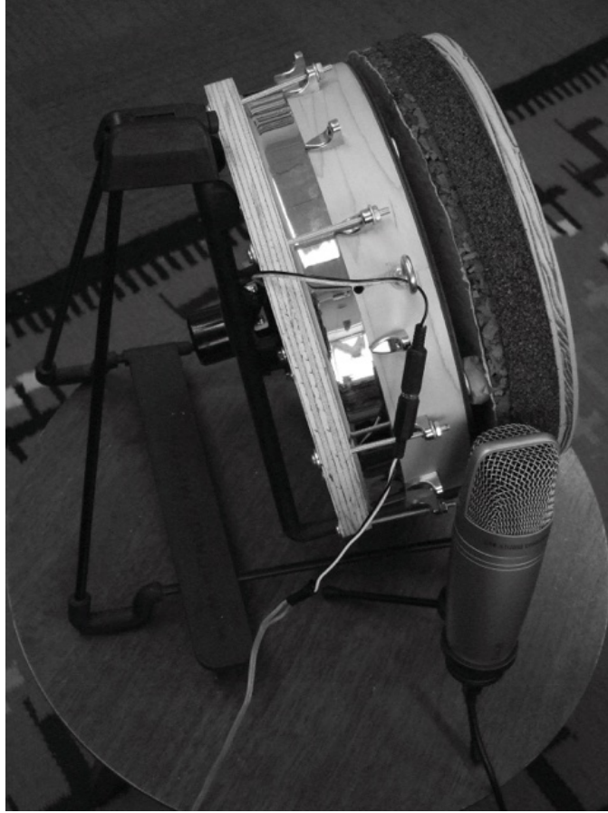
FIG. 12. wood “head” with 3” speaker and cork & foam belly-back
