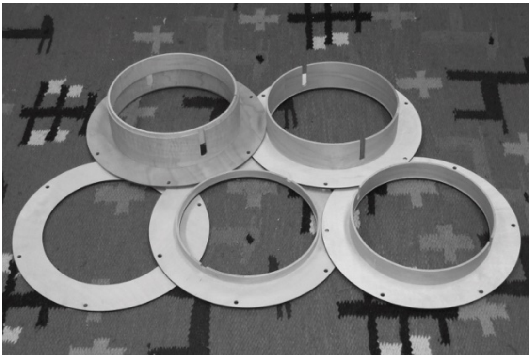
FIG. 13. internal resonators of various and variable heights
