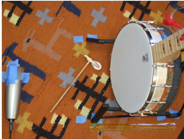
FIG. 15. microphone on the floor to record head taps on the shallow rim with the belly back
