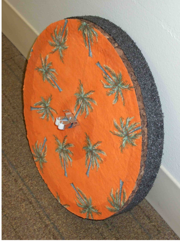
FIG. 4. The synthetic belly: 1" closed-cell foam, 5/8" cork, & cotton Hawaiian shirt
