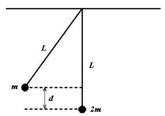
A pendulum of mass  $m_1 = m$  is raised a distance d and dropped so that it collides elastically with a second pendulum of mass  $m_2 = 2m$ .
